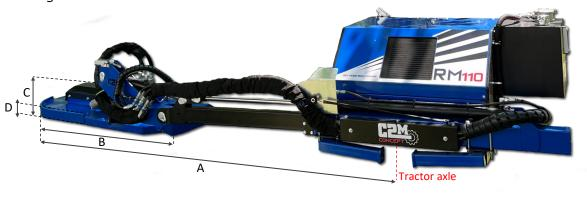
A) Max. length unfolded: 3000mm and min. length folded: 2100mm B) Cutting head length: 1100mm
